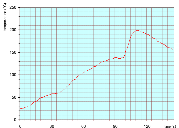
Example of a measured preheating profile
